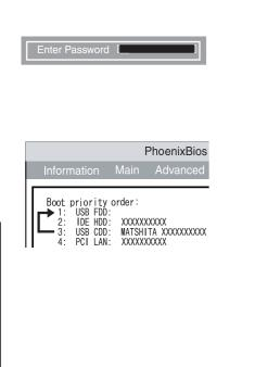
Turn the computer on, and press the **F2** key while [Panasonic] boot screen is displayed.
